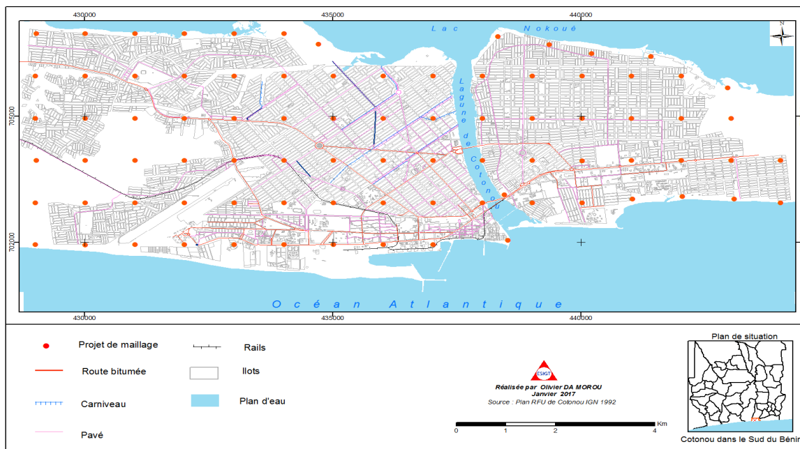
Figure-1: Project of theoretical grid of 1 km of the points to be determined with the GNSS and the direct leveling on the city of Cotonou 3 .
