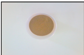
Figure-2: Prepared adsorbent material (TR); particle size: <150\mu\text{m}
