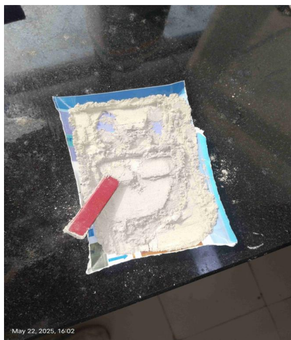
Figure-1: Coal Fly Ash Treatment with Bar Magnet.
