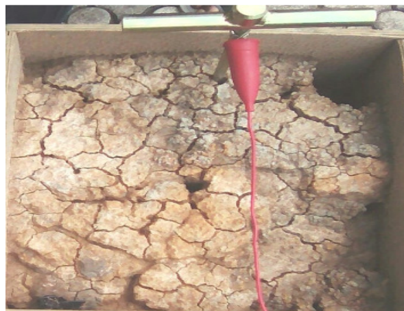
Figure-2: Kaolinite clay undergoing resistivity test.
