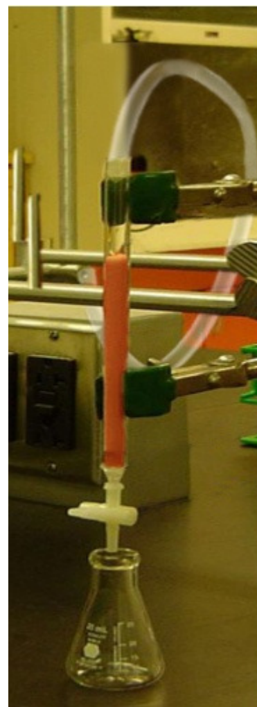
Figure-1 Photograph showing the experimental set up for fixed-bed column study
