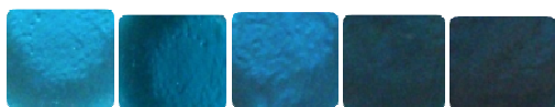
Cu-1% Cu-2% Cu-3% Cu-4% Cu-6% Photographs of Cu ion doped investigated glass samples
