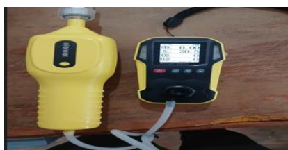
Figure-3: Biogas analyzer to determine the composition of the biogas produced during the experiment.
