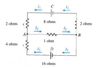
There are two batteries and four resistors in this electrical network. Moreover, Current I<sub>1</sub> flows through the top branch BCA, Current I2 flows across the middle branch AB and Current I<sub>3</sub> flows through the top branch BDA. By the Current law we get  $I_1 - I_2 + I_3 = 0$  at node A. We also obtain the same equation at node B.
