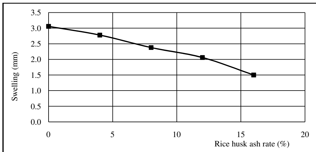
Figure-5: Swelling evolution according to rice hush ash rate.
