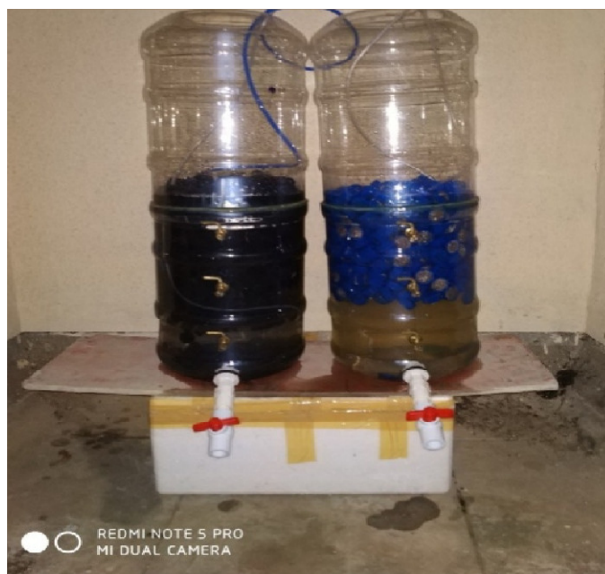
Figure-7: Domestic waste water treatment unit with FAB media and water bottle caps media.
