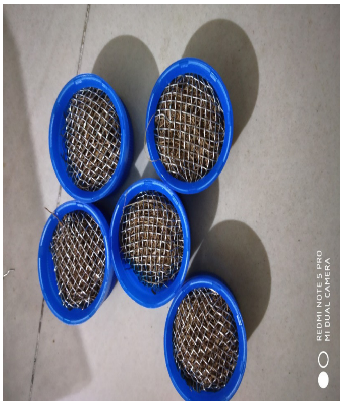
Figure-4: Prepared water bottle cap media with coir and sealed with mesh.
