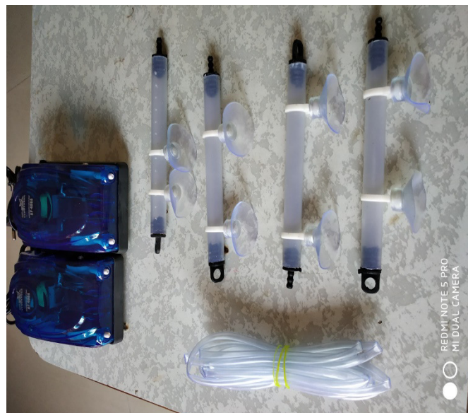
Figure-6: Material used for aeration like air pump, pipe and diffuser.
