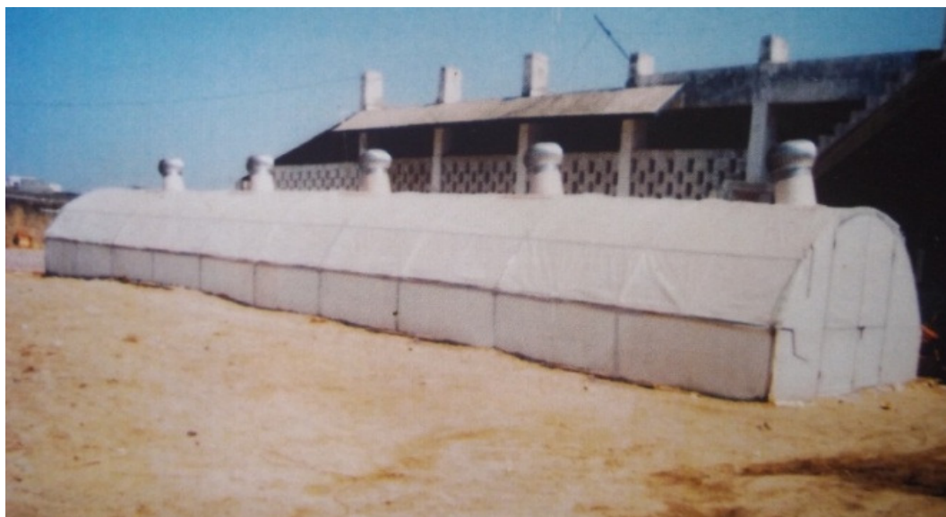
Figure-2 Greenhouse type solar tunnel dryer installation
