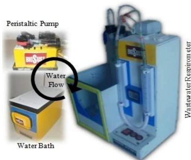
Figure-1 'BIOSUST' differential respirometer integrated with a water bath and peristaltic pump
