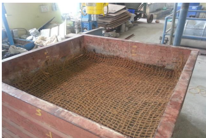
Figure-3b: Tank setup with geotextile layer.
