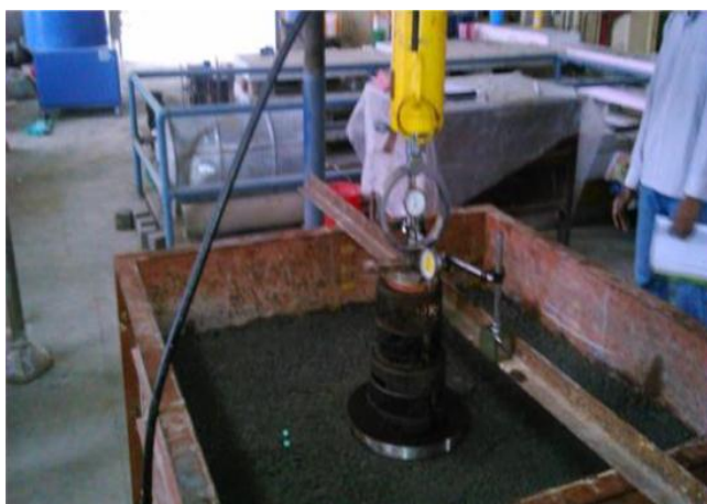
Figure-3a: Plate load test setup on subgrade.
