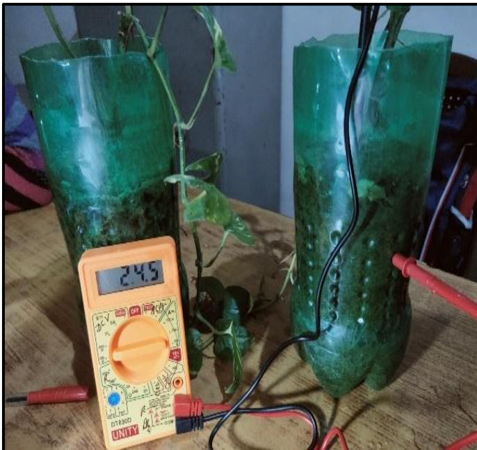
Figure-2: Experimental setup of a plant-based nano power plant using Epipremnum aureum to generate electricity via root-zone microbial activity.
