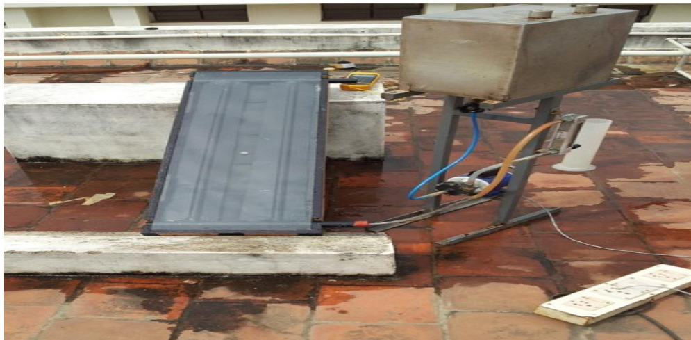
Figure-11 Experimental Setup of the solar collector
