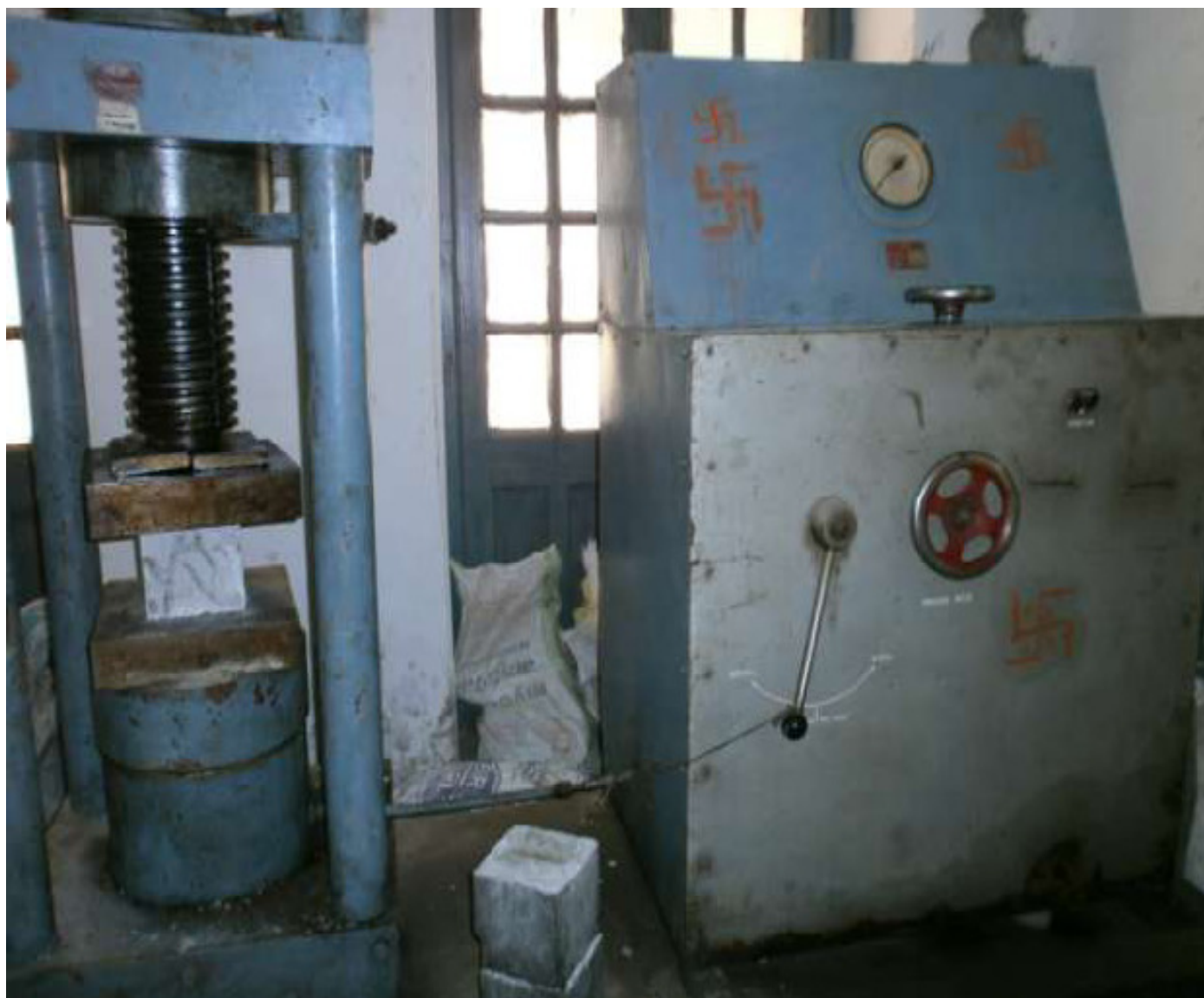
Figure-1 Testing of concrete cube in testing machine
