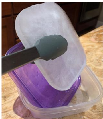
Figure-5: After melting for 5 minutes, ice blocks were gently shaken for 15 seconds with silicone tongs.
