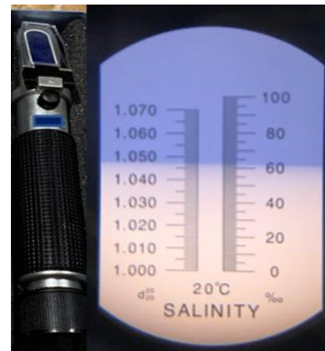
Figure-3: Salinity was measured with an aquarium saltwater refractometer.
