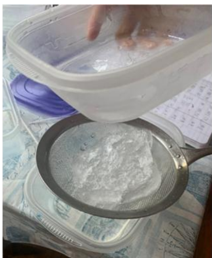
Figure-2: Contents of container were placed in a strainer to separate ice shards from brine every 5 minutes.
