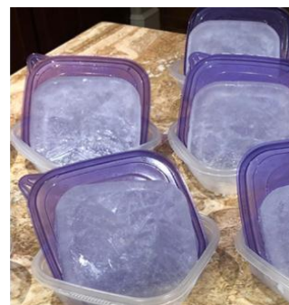
Figure-4: Containers were removed from freezer and ice blocks were tilted and melted at 22.8 degrees Celsius.
