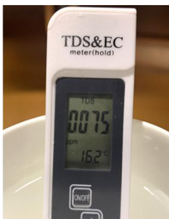
Figure-6: Total dissolved solids (TDS), for product water as well as tap water were measured.
