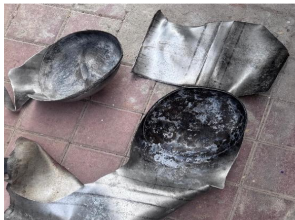
Figure-1: Remnants of exploded cylinder.
