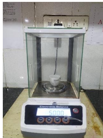
Figure-1: Weighing of a 5g shilaith sample.
