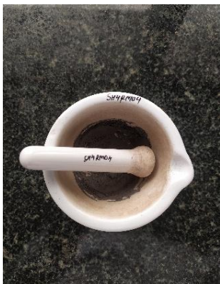
Figure-4: Crushing and homogenization into a fine powder.
