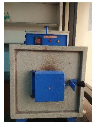
Figure-3: Dry ashing of the sample.
