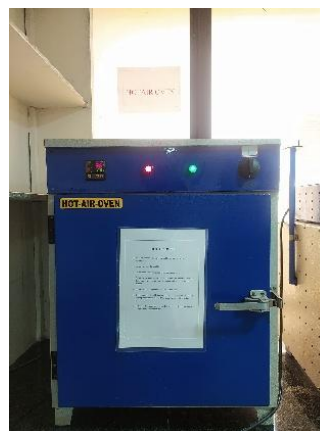
Figure-2: Drying of the sample at 60 ° C in a hot air oven.
