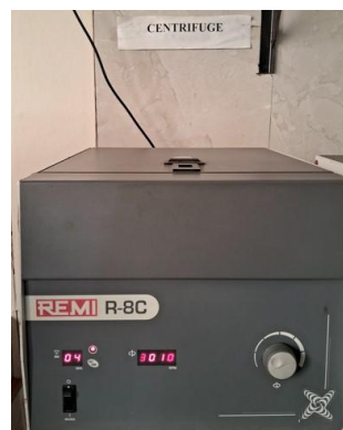
Figure-3: Centrifugation of the mixture for 5 minutes at 3000 rpm.
