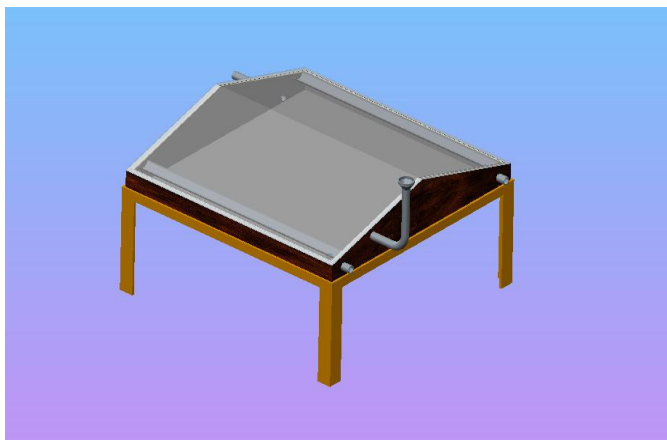
Figure-3 Proposed model of solar distillation system
