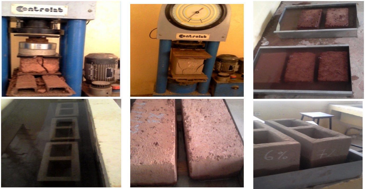
Figure-7: Compression, Immersion and capillary absorption (a) Compression of laterite bricks; b) Compression of cinder blocks; c) Immersion of laterite bricks, d) Immersion of cinder blocks, e) Capillary suction of laterite bricks, f) Capillary suction of cinder blocks.
