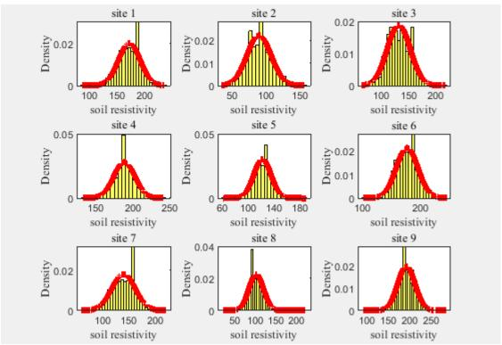
Figure-5: Soil electrical Resistivity distribution.
