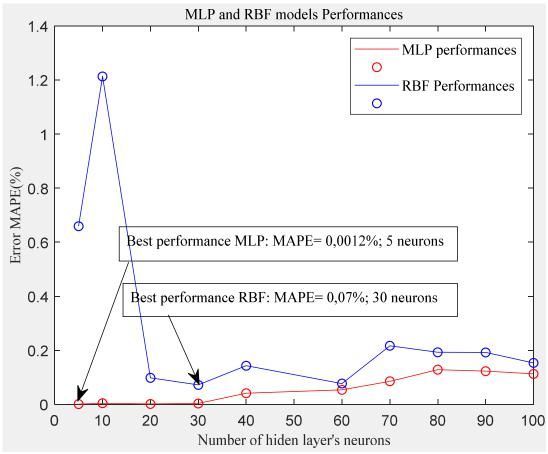
Figure-6: MAPE error according to the number of hidden layer's neurons for MLP and RBF.
