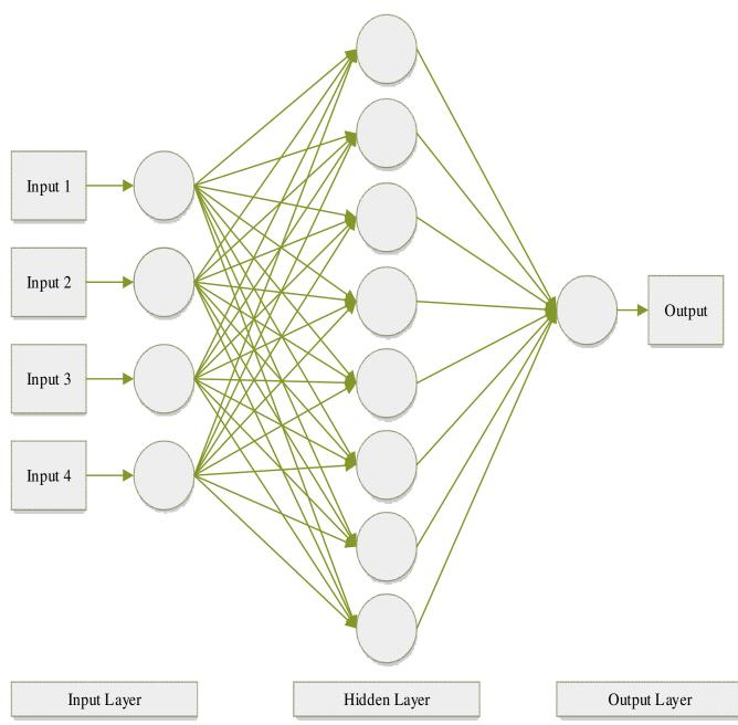
**Figure-1:** Structure of two layers ANN<sup>10</sup>.
