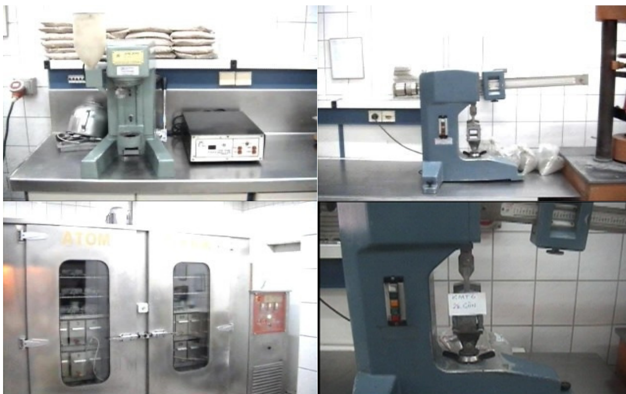
Figure-2: Equipment for preparation and testing of mortar composite, left to right, the automatic-minute-controlled mixer, the bending moment testing machine, curing cabinet whose relative humidity and water temperature is controlled by computer, bending moment testing of mortar composite containing MP.
