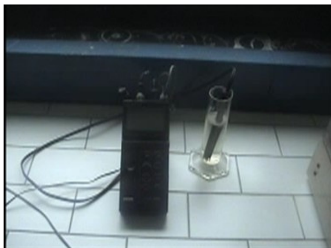
Figure-1: Image of pH meter for measuring of cement alkalinity.
