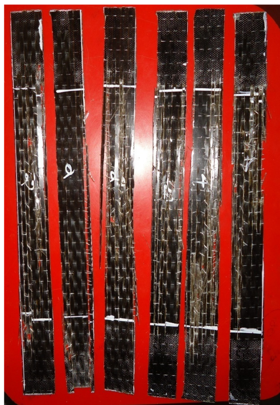
Figure-6 Failure specimens for 90 0 orientation
