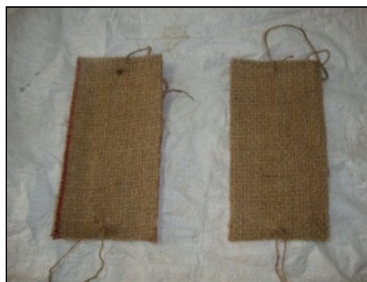
Figure-1 Jute samples ready for impregnation with bitumen
