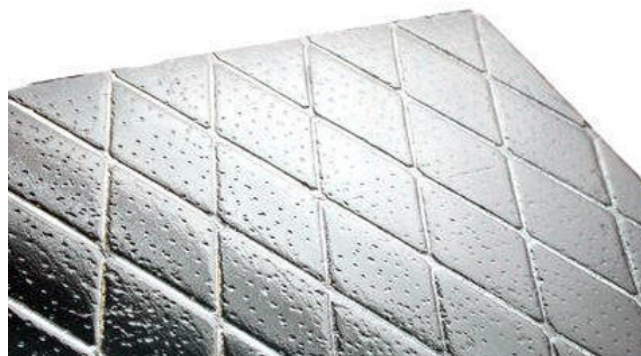
Figure-8 An example of the VIP- Vacuum insulation panels
