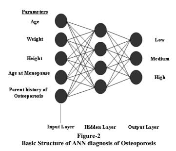
Normally, multilayer perceptron uses backpropogation learning algorithm. These algorithms minimize the error between desired value and output value by using recursively delta rule. Backpropogation calculate error, compute delta (difference), propagate error backwards and then update the weights. After updating, these weights feed in training patterns. Figure-3 shows the major steps to be followed for building ANN for predicting fracture risk.
