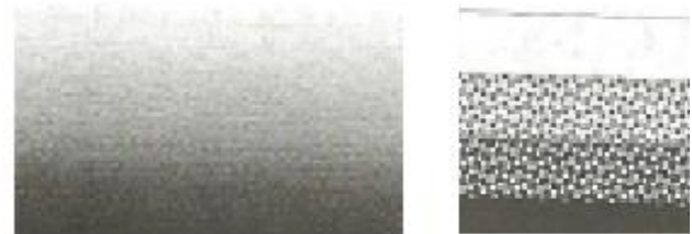
Figure 1 Continuous and Stepwise graded structures 1
