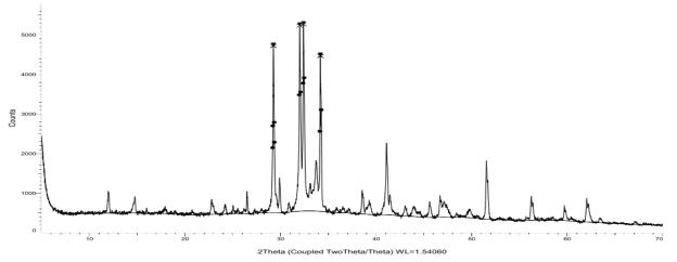
Figure-4 X-Ray Diffraction for post peak analysis of OPC
