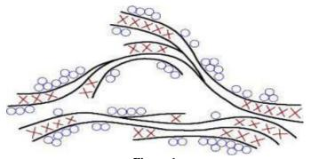
Figure-1 Feldman-Sereda model for the microstructure of C-S-H Black lines: C-S-H sheet, Circles: Adsorbed water, Crosses: Interlayer water
