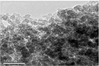
Figure- 2 TEM image of nano SiO<sub>2</sub>
