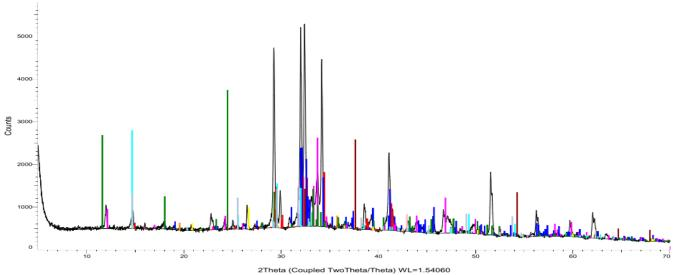
Figure-3 X-Ray Diffraction of Ordinary Portland Cement [OPC]
