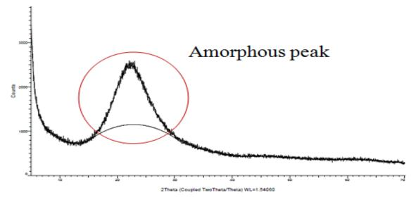
Figure-3 X-Ray Diffraction of nano SiO<sub>2</sub>
