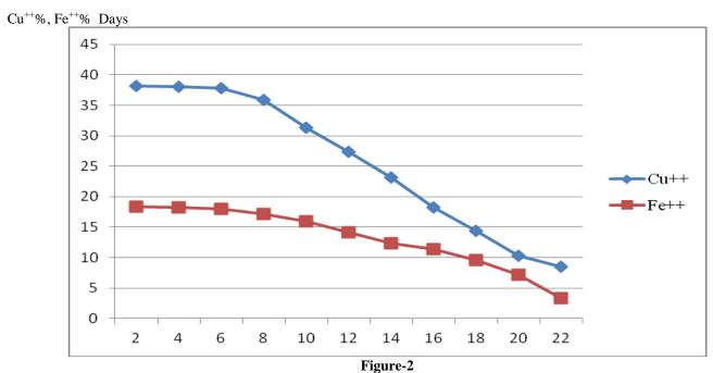
Course of metal extraction during bioleaching process using Bioreactor
