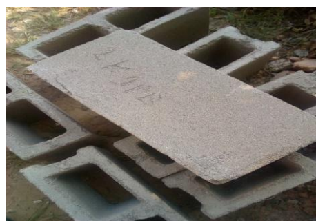
Figure-4: Hollow bricks of 2% P. biglobosa sawdust replacement for sand.
