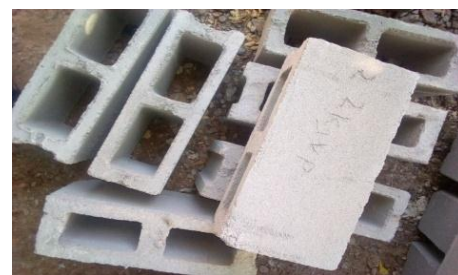
Figure-5: Hollow bricks of 2% V. paradoxa sawdust replacement for sand.
