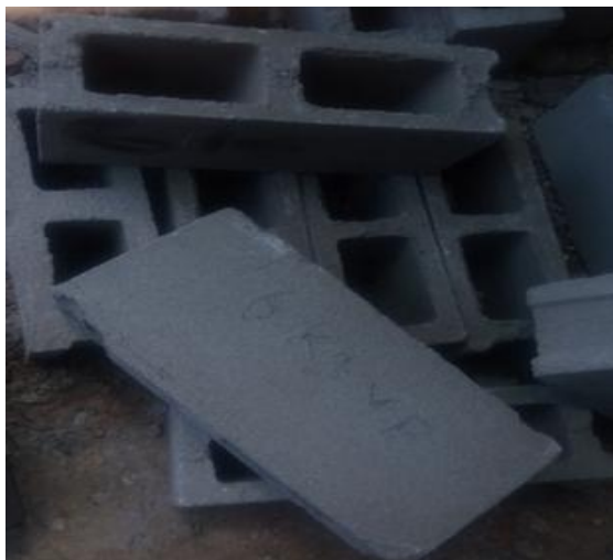
Figure-9: Hollow bricks of 6% V. paradoxa sawdust replacement for sand.
