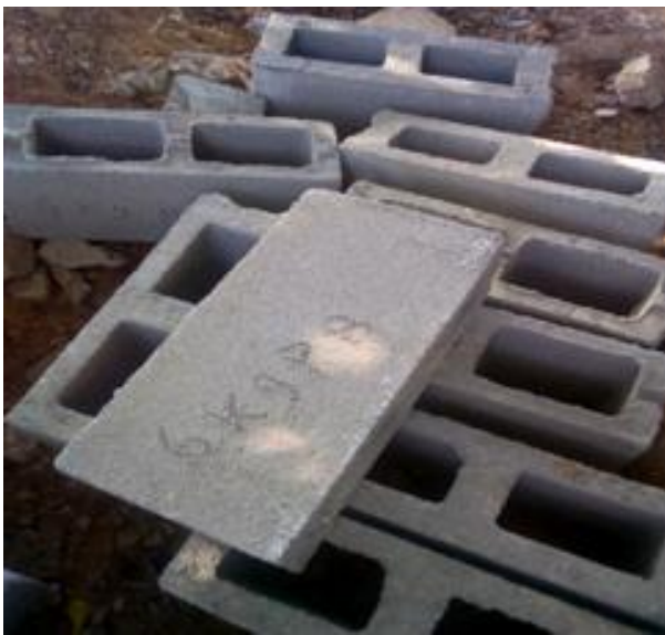
Figure-8: Hollow bricks of 6% P. biglobosa sawdust replacement for sand.
