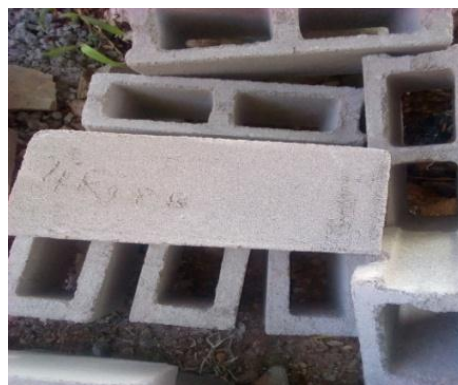
Figure-6: Hollow bricks of 4% P. biglobosa sawdust replacement for sand.
