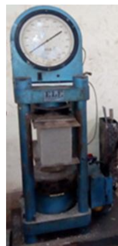
Figure-3: Brick compressive strength test in the laboratory.
