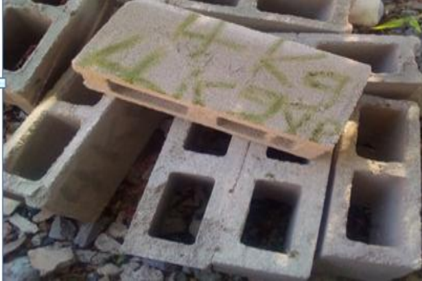
Figure-7: Hollow bricks of 4% V. paradoxa sawdust replacement for sand.
