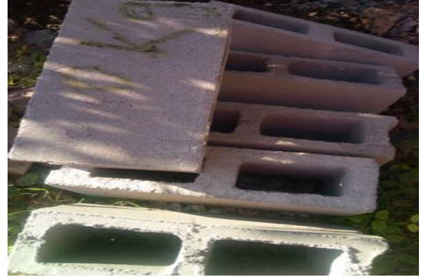
Figure-10: Hollow bricks of 0% sawdust replacement for sand.
