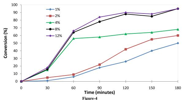
Influence of mass ratio of CaO concentration on transestrification of simarouba oil, Oil/Methanol molar ratio is 1:12, Reaction temperature is 65<sup>0</sup>C
