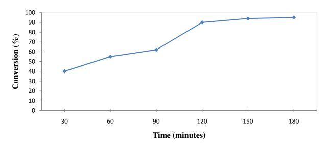
Figure-5 Influence of reaction time on transestrification of simarouba oil, CaO/oil mass ratio is 8%. Oil/methanol molar ratio is 1:12, Reaction temperature 65<sup>0</sup>C
