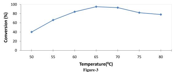
Influence of reaction temperature on transestrification of Simarouba oil, CaO/oil mass ratio is 8%, Oil/methanol molar ratio is 1:12, Reaction time is 180 minutes
