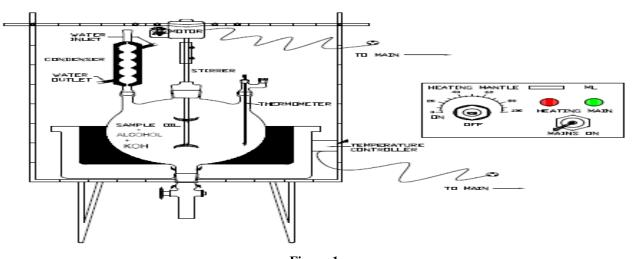
Figure-1 Schematic diagram of a transestrificator (from Mishra et.al., 2012)<sup>3</sup>
