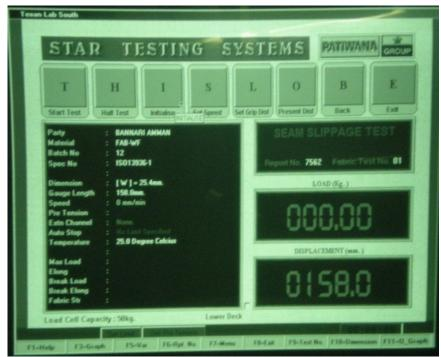
Figure-2 Parameter Setting Screen for Fabric Testing
