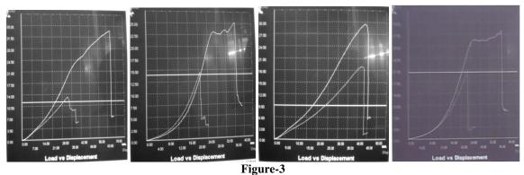
Load-Displacement curve for polyester-cotton plain unfinished and finished fabric at warp and weft direction
