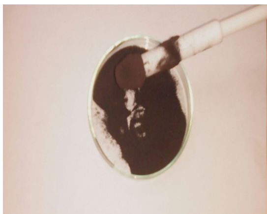
Figure-5: (b) MIONAC attracted by magnetic retriever.
