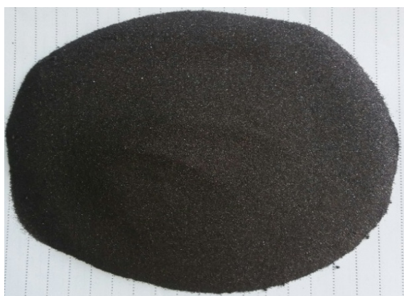
Figure-1: Sample of titaniferous sand used as an adsorbent.
