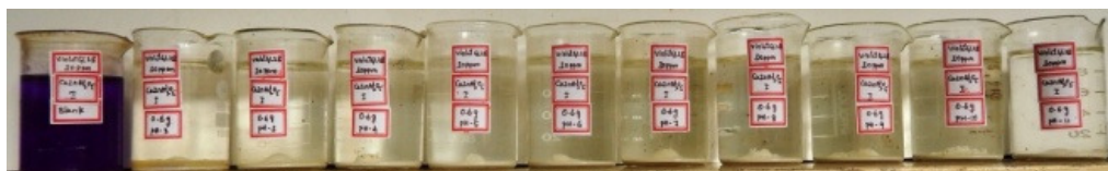
Figure-10 Effect of pH on VGL2B at 120 minutes [VGL2B =30 mg/L, \text{CaZnAl}_2\text{O}_5 = 0.6g/100ml]
