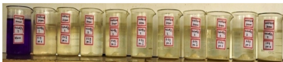
Figure-8 Effect of catalyst concentration on VGL2B at 120 minutes [VGL2B =30 mg/L, pH=7]
