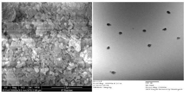
Figure-4 SEM and TEM micrograph of SZM at Crystallization Temperature of 150°C
