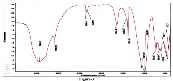
FTIR Spectrograph of SZ at Crystallization Temperature of 200°C
