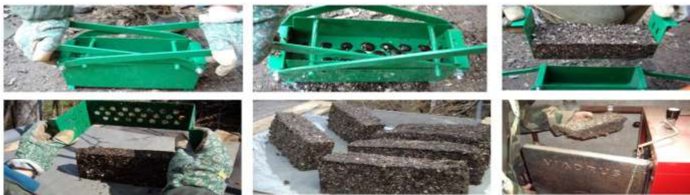
Figure-1 Technology for producing sapropel and sawdust briquettes
