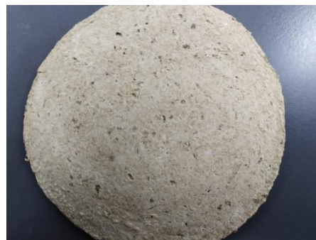
Figure-5: The color of the paper is lightened due to the presence of CaCO 3 nanoparticles.
