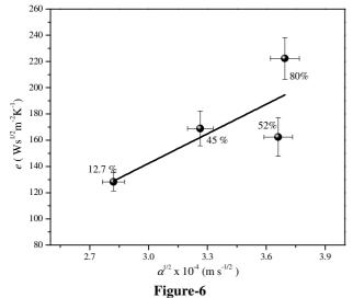
Thermal effusivity as a function of the square root of the thermal diffusivity for samples taken from the top culm region of the Guadua for different moisture contents, the solid line is the best least squares linear fit whose slope is equal to the volume specific heat,  $\rho C$
