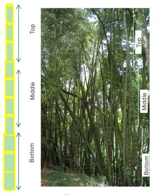
Figure-1 The Guadua culm was divided in three zones through its longitude: bottom, middle and top
