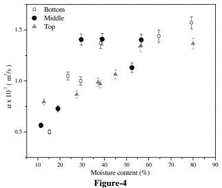
Thermal diffusivity values as a function of moisture content for three longitudinal sections of the Guadua: bottom, middle and top
