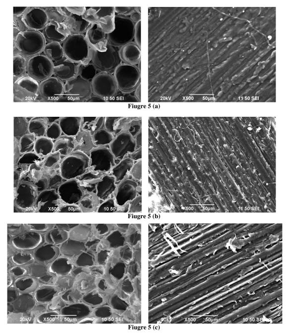
SEM micrographs of samples taken from: (a) bottom, (b) middle and (c) top of longitudinal zone in Guadua with 11.8% moisture content. The three images showed on the top correspond to a cross-section view while those of the bottom are photographs of a lateral view
