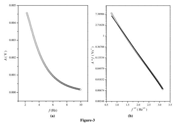
(a) Typical curve of the PA signal amplitude (A) as a function of the modulation frequency (f) for a sample with 11.8 % of moisture content taken from the middle zone of *Guadua* culm. (b) Logarithm of the A\*f product plotted as a function of the square root of the modulation frequency for the same sample considered in (a). The solid line corresponds to the best least squares linear fit as given by the Rosencwaig-Gersho model for an opaque and thermally thick sample (Eq. (2))
