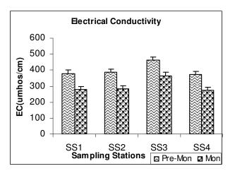
Fig-2: Graph showing variation in Electrical conductivity Concentration at different sampling stations
