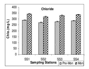
**Fig-9:** Graph showing variation in Chloride Concentration at different sampling stations
