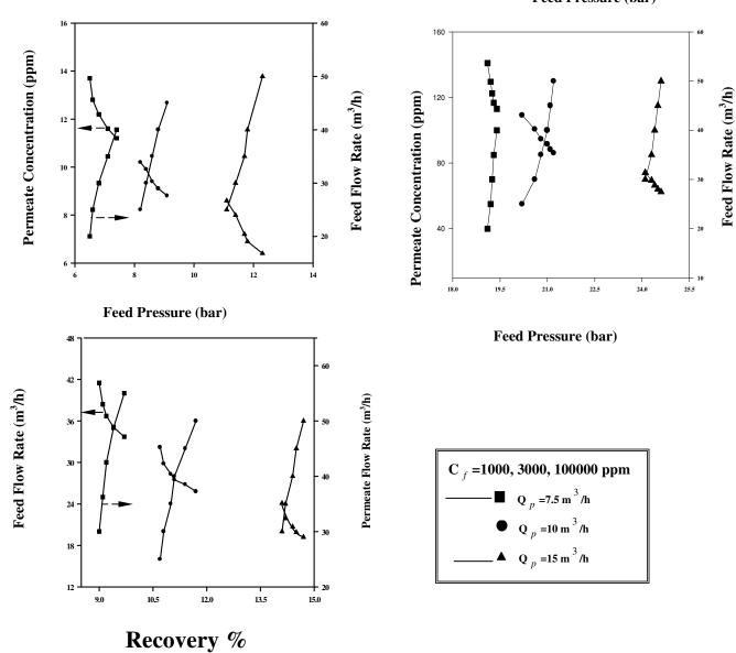
Figures-5, 6 and 7: show the Influence of feed pressure and feed flow rate on the optimum concentration of permeate water with various feed water concentration.
