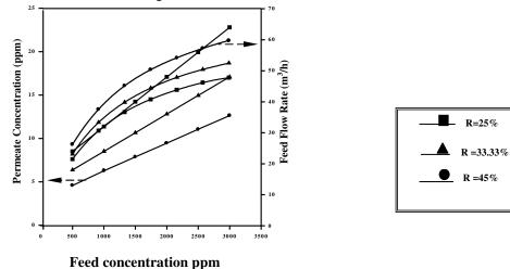
Figure-4: Influence of feed concentration and feed flow rate on the optimum concentration of permeate water
