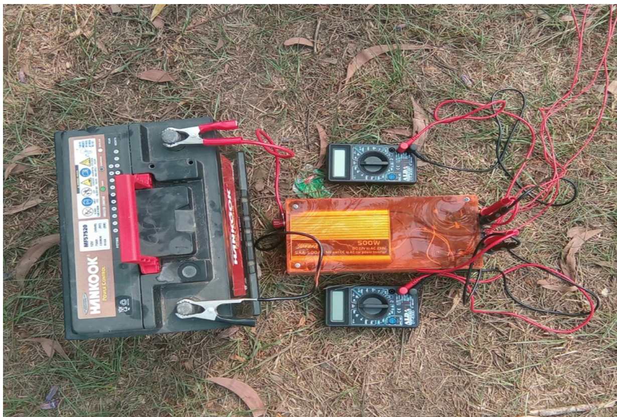
Figure-2: The constructed simple resistivity meter and its components.
