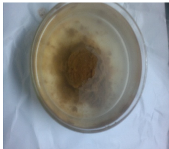
Figure-4 Crumb test result for Bentonite (after six hours)
