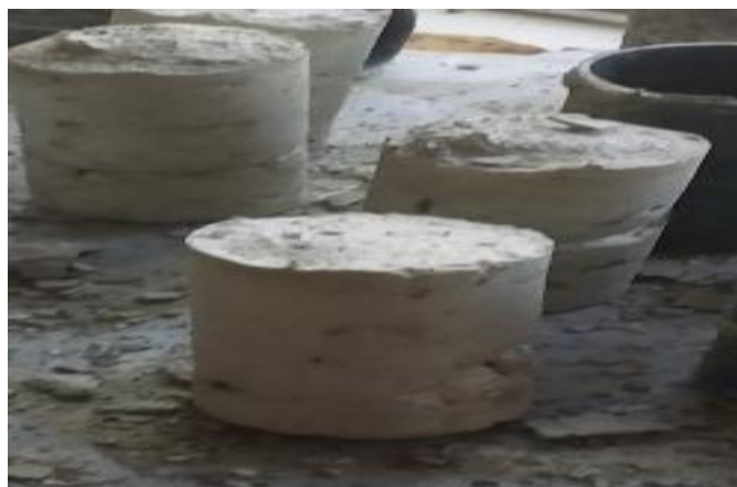
Figure-4: Core samples produced from sandstone.
