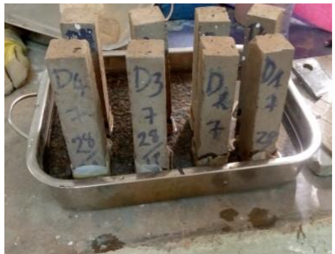
Figure-6: Device of water absorption of the specimens.
