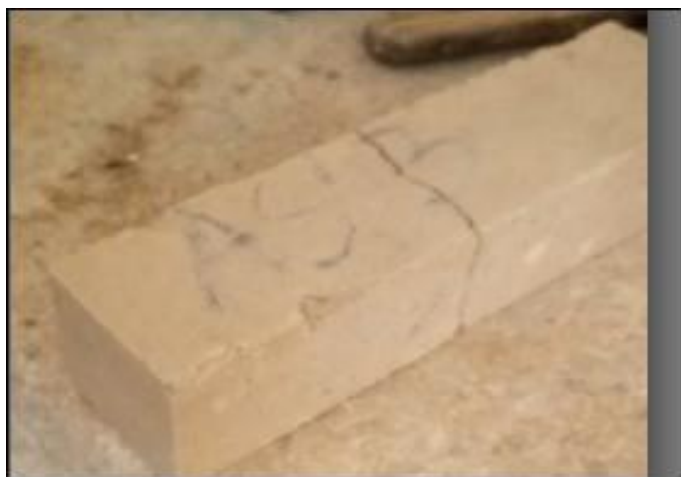
Figure-8: Rupture of a specimen in two parts.
