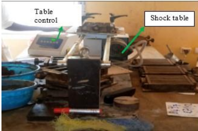
Figure-4: Device for the production of adobes.
