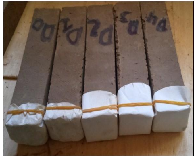
Figure-5: Placing of filter papers.
