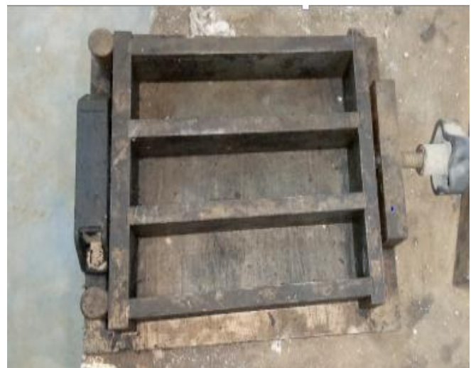
Figure-3: Metal mold used to make adobes.
