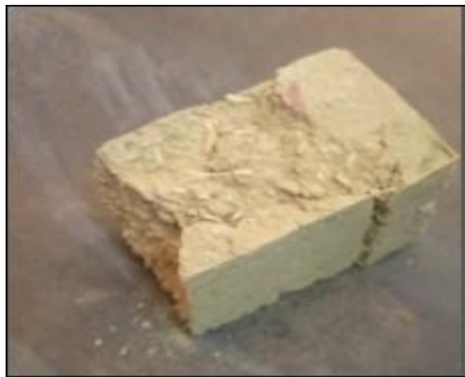
Figure-10: Adobe crushed by compression.
