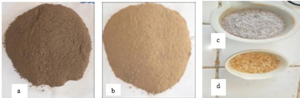
Figure-1: a- MOD clay soil sample, b- NDJA clay soil sample, c- burnt rice husk, d- unburnt rice husk.
