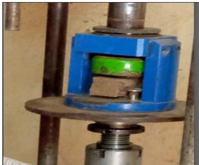
Figure-9: Device for compressing adobes.
