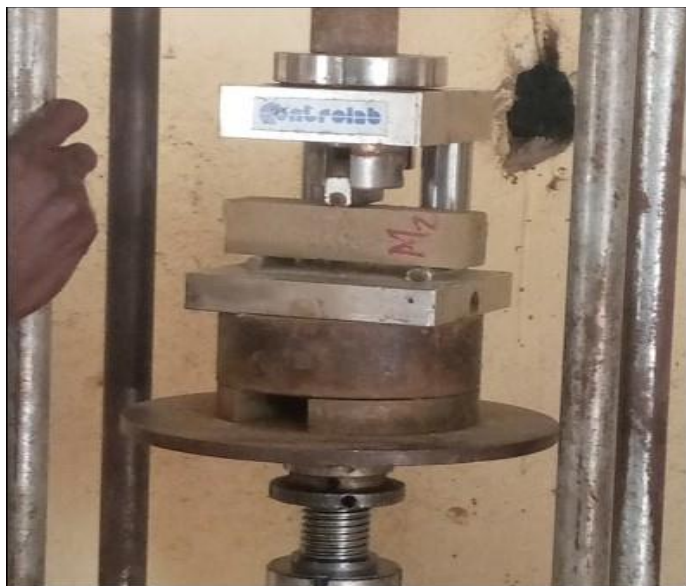
Figure-7: 3-point flexing device.
