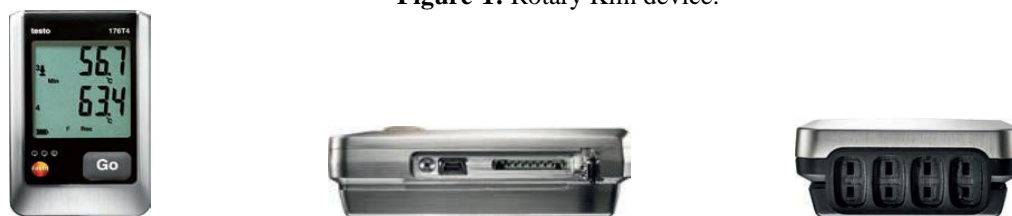
Figure-2: Testo 176T4 with interface USB, SD card and thermocouples probe.
