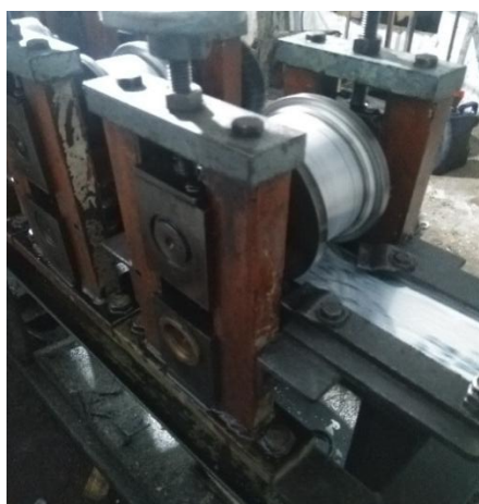
Figure-2: Rolling mill used for shaping thin strip into channel.
