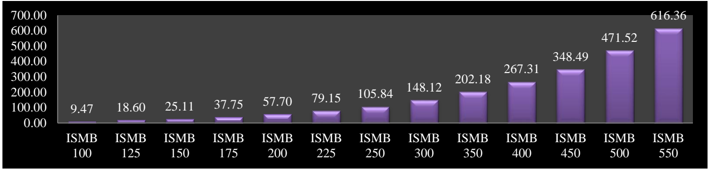
Figure-2: Design bending moment of ISMB sections.
